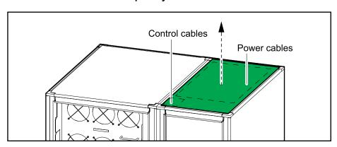
10. Drill holes and install conduits for power cables and for control cables in the top gland plate. Conduits are not provided.
