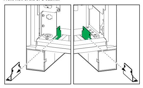
5. **For bottom cable entry only**: Drill holes and install conduits for power cables and for control cables in the bottom of the rear part of the conduit box. Conduits are not provided.
