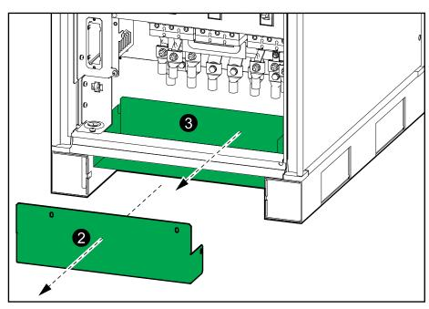
4. Remove the indicated brackets in the right and the left side of the UPS cabinet. Discard the brackets, but save the screws for installation.
