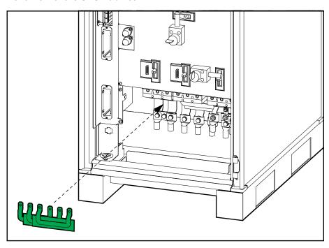
Front View of the UPS Cabinet with the Busbar Assembly for Single Mains Installed
