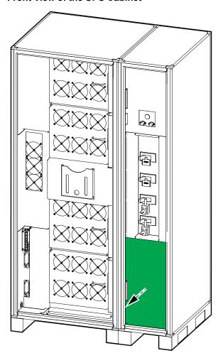
2. Remove the gland plate in the top or bottom of the I/O section.
