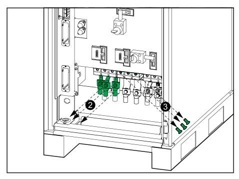
4. Install the provided busbar assembly for single mains between the unit input breaker UIB and the static switch input breaker SSIB and fasten with the six busbar screws removed in earlier steps.
