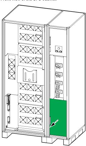
2. Install the three provided jumper busbars between the input busbars and the bypass busbars.
