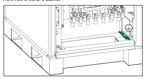
3. Connect the input cables to the input terminals (L1, L2, L3 (N)).
