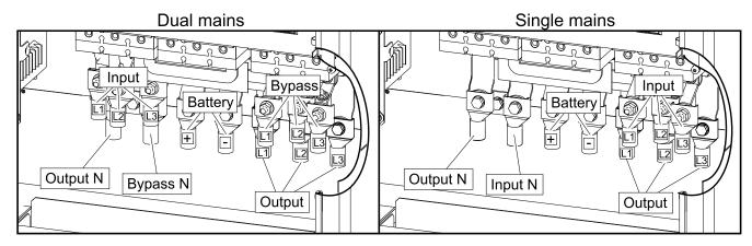
4. Connect the bypass cables to the bypass terminals (L1, L2, L3, N).
