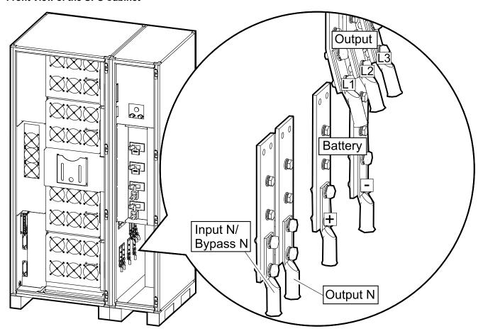
10.**Only for configurations with adjacent battery cabinet(s)**: Route the battery cables (+,-, ground) through the left side panel and connect them to the battery busbars (+, -) and the ground busbar in the power section.
