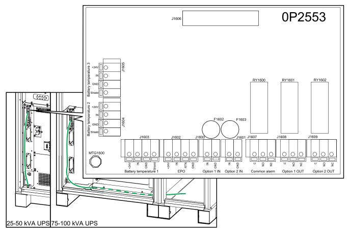
2. Connect the signal cables to the input contacts and output relays on the external connection board 0P2553.
