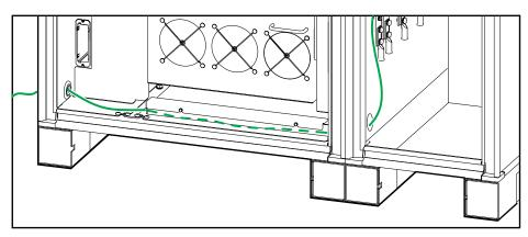
3. Connect the control cables from the control terminal block TB1 in the battery cabinet(s) or the battery breaker box to the control terminal block TB1 in the UPS cabinet as shown.
