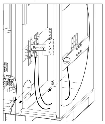
6. **Only in single mains configurations**: Remove the three preinstalled bypass cables in the right side of the top entry cabinet.
