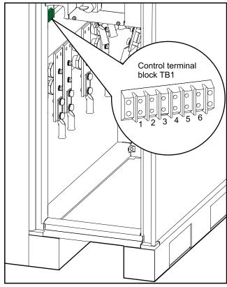
2. Only for configurations with adjacent battery cabinet(s): Route the control cables through the left side panel of the 25-50 kVA UPS or through the cable channel in the power section on the 75-100 kVA UPS to the control terminal block TB1.
