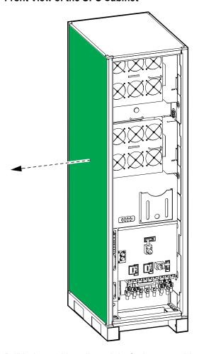
3. Drill holes and install conduits for battery cables and for control cables in the side panel. Conduits are not provided. Fit the holes to the placement of the cable inlets inside the UPS cabinet.
