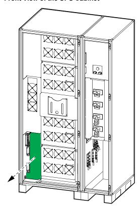
2. Remove the side panel from the power section of the UPS cabinet.
