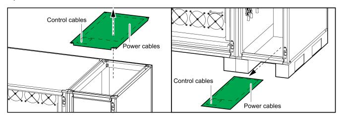
3. Drill holes and install conduits for power cables and for control cables in the gland plate. Conduits are not provided.
