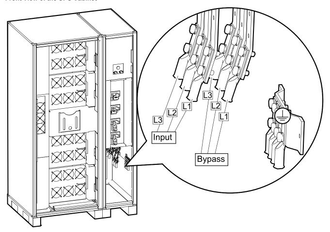
8. Route the output cables through the top or bottom of the I/O section and connect the output cables to the output terminals (L1, L2, L3, N). The neutral cable connects in the left side of the I/O section.
