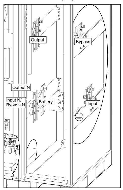
17. Route the input cables through the top gland plate and connect to the input busbars (L1, L2, L3, (N)) in the top entry cabinet.
