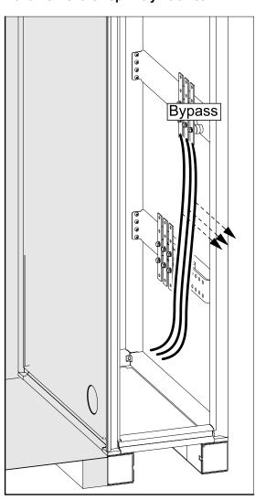
7. Install two interconnection brackets on the front of the cabinets and two interconnection brackets in the rear of the cabinets. Use C-clamps to hold the cabinets together to make the installation easier. Use four screws on each side of each interconnection bracket to fasten it to the cabinet frame.
